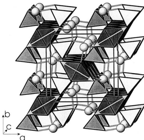
**Fig. 7** Polyhedral drawing of the structure of kanonaite. Jahn-Teller elongated  $\text{Mn}^{3+}$  octahedra (light arrows indicate the direction of elongation) form edge-sharing chains parallel to the  $c$  axis. Al (spheres with bonds) prefers distorted trigonal bipyramidal coordination forming edge-sharing dimers
