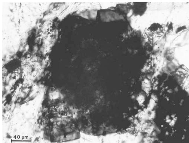
**Fig. 2** Transmitted-light photograph of largely opaque kanonaite aggregate (centre) in sample Cor 8-1. Only towards the rims (top, lower left, right) can some small transparent kanonaite crystals be recognized. Along its upper left edge, the opaque kanonaite is surrounded by an elongated aggregate of small flakes of muscovite and additional opaques
