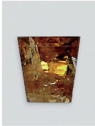
Figure 2. The 0.23 g hibonite crystal (left) was fashioned into a 0.39 ct step-cut gem (right). The smooth surface on the rough is a polished facet, which corresponds to the table of the faceted gem. The c -axis is nearly vertical. Photos by T. Hainschwang (left) and F. Notari (right).
